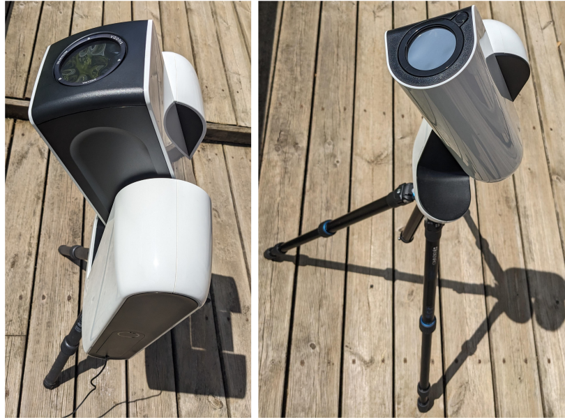
Fig. 2: A Stellina (left) and a Vespera (right) smart telescopes, with dedicated solar filters.
