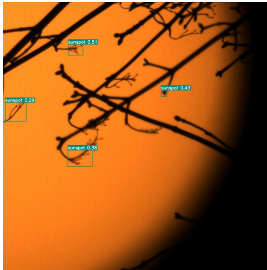
Fig. 1: Solar image captured with a Vespera smart telescope (16/1/2024) and annotated with a YOLOv5 detection model presented in [14]: the models detect trees as sunspots – these are false positives.
